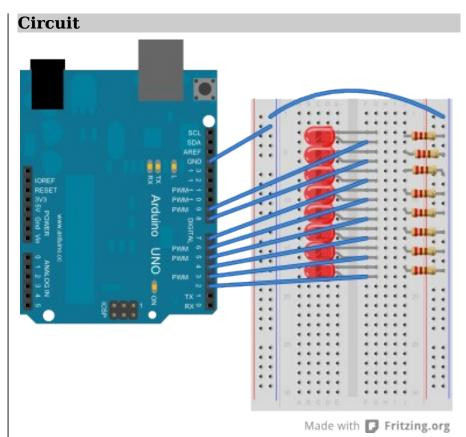
**NOTES:** You are connecting the Arduino pins to the anodes (long lead) of the LEDs. The cathodes (short lead) connect to a  $220\Omega$  resistor that connects to ground (blue rail). Don't forget to connect the GND pin from the Arduino to the blue ground rails!
